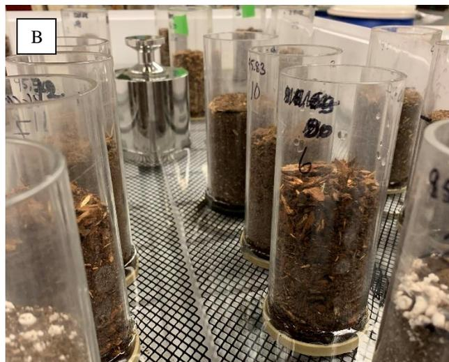
Figure 1: A) Photograph of the NCSU Wettability Manual setup with beakers collecting effluent from cylinders after an irrigation event and B) Subirrigated samples in an Ebb and Flood table during an irrigation event.
