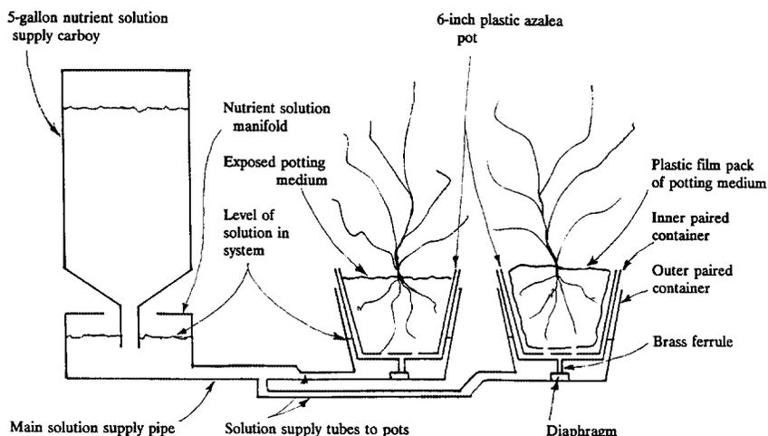
Figure 1. Stylized diagram of potted plant subirrigation system.
