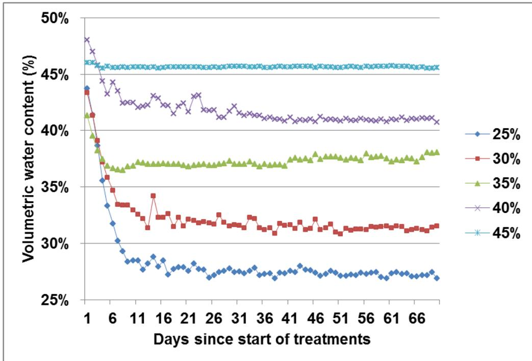
Figure 1. Daily average substrate volumetric water content maintained by a soil moisture sensor-controlled automatic irrigation system.
